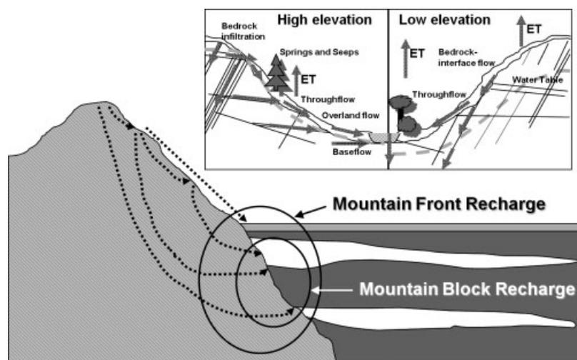
Figure 1. Conceptual diagram for MFR and MBR. Insert diagram depicts upland subcatchment routing of precipitation that may include discharge of groundwater to streamflow and subsequent streamflow loss to groundwater recharge via channel seepage
