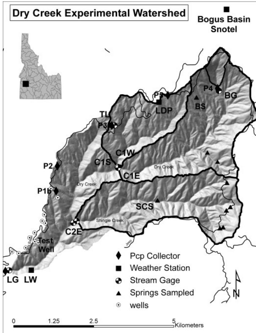
Figure 2. DCEW. Measurement site instrumentation is shown with study catchments outlined as defined by outlet measurement points LG, C2M, C2E, C1E, C1W, TL, and BG. Springs C1S and SCS are also identified
